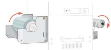
When the drawer comes out the thermo sealing film unfolds and **C26S after 12 seconds from the cycle** beginning is ready again to pack in MAP.
